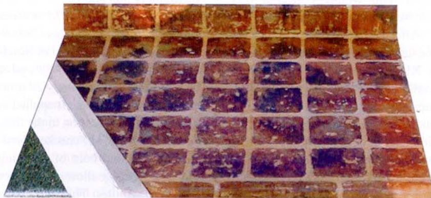
This cutaway section shows the layering of Formica, XIM, Bonding Primer, Overlay and Stain.
